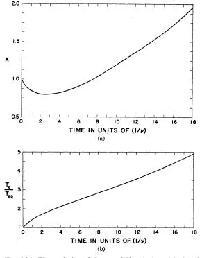
FIG. 9(a). The variation of electron drift velocity with time for  $E/E_c=0.2$ . The initial conditions are x(0)=1.0 and  $T_e(0)=T_{e0}$ . (b). The variation of electron temperature with time for  $E/E_c=0.2$ . The initial conditions are x(0)=1.0 and  $T_e(0)=T_{e0}$ .
