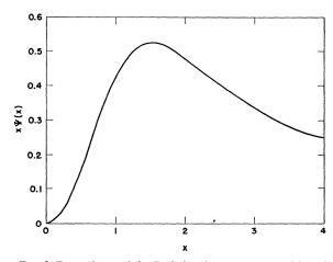
FIG. 3. Dependence of the Joule heating rate expressed in units of  $eE_c\beta_e^{-\frac{1}{2}}$  upon the relative electron-ion drift velocity. The latter is expressed in units of the most probable random electron speed,  $\beta_e^{-\frac{1}{2}}$ .
