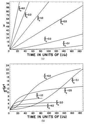
FIG. 4(a). The variation of electron drift velocity (expressed in units of  $\beta_e^{-\frac{1}{2}}$ ) with time for a range of the parameter  $E/E_c$ . The initial conditions are x(0) = 0 and  $T_e(0) = T_{e0}$ . (b). The variation of electron temperature (expressed in terms of the initial temperature  $T_{e0}$ ) with time for a range of the parameter  $E/E_c$ . The initial conditions are x(0) = 0 and  $T_e(0) = T_{e0}$ .
