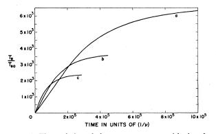
FIG. 8. The variation of electron temperature with time for  $E/E_e=0$ . The initial and final conditions shown are: (a) x(0) = 100,  $T_e(0) = T_{e0}$ ,  $x(10^6) = 24$ ; (b) x(0) = 75,  $T_e(0) = T_{e0}$ ,  $x(4.6 \times 10^5) = 15$ ; (c) x(0) = 60,  $T_e(0) = T_{e0}$ ,  $x(2.8 \times 10^5) = 8$ .
