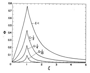
FIG. 10. The variation of the dynamical friction function  $\Phi(\xi,\zeta)$  with the electron drift velocity for a range of values of the anisotropy parameter  $\zeta$ .
