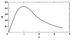
FIG. 1. The variation of the dynamical friction function  $\Psi$  with the relative electron-ion drift velocity (expressed in units of  $\beta_{e}^{-\frac{1}{2}}$ ).
