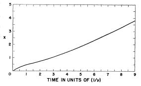
FIG. 7. The variation of electron drift velocity with time for  $E/E_e = 0.6$ . The initial conditions are x(0) = 0 and  $T_e(0) = T_{e0}$ .
