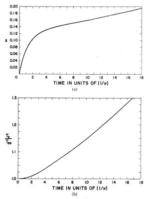
FIG. 5(a). The variation of electron drift velocity with time for  $E/E_c=0.1$ . The initial conditions are x(0)=0 and  $T_e(0)=T_{e0}$ . (b). The variation of electron temperature with time for  $E/E_c=0.1$ . The initial conditions are x(0)=0 and  $T_e(0)=T_{e0}$ .
