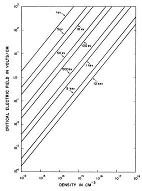
FIG. 2. Critical electric field,  $E_c$ , as a function of the particle density with the average electron energy,  $\frac{3}{2}kT_e$ , treated as a parameter. The cutoff factor,  $\ln(\lambda/p_0)$ , was assumed to be 10 for all conditions.
