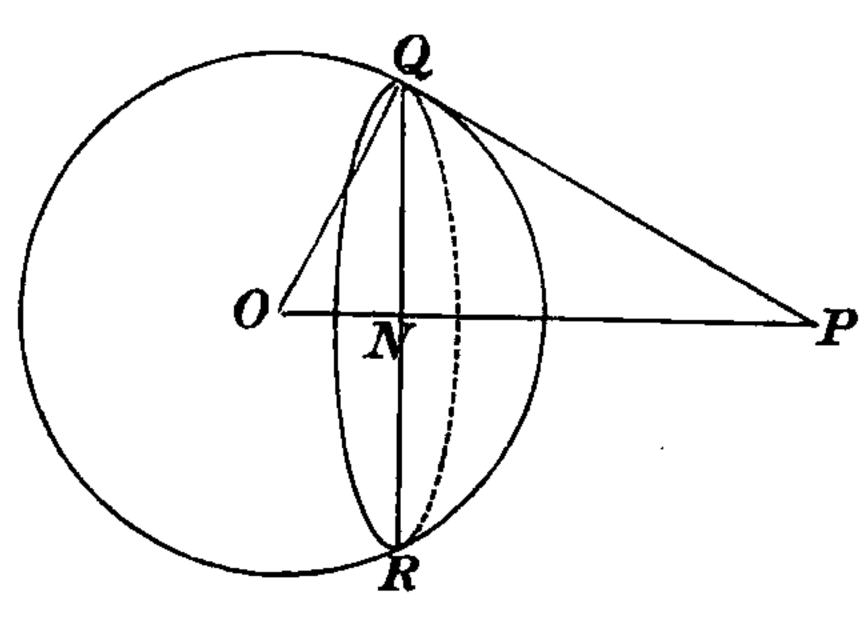
$2\pi a^2 \sin \theta d\theta$ . Hence if M be the mass of the shell, the component attraction of the band on P, along PO, is
