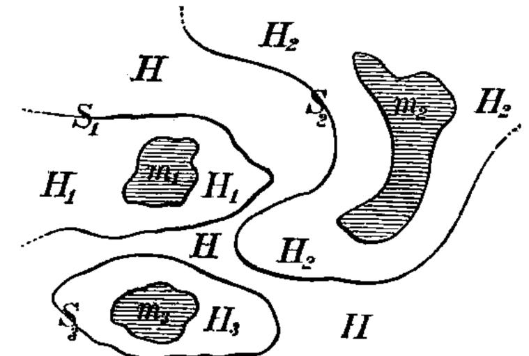
one, distribution of matter over S, which shall produce the potential of  $m_1$ , throughout all the space  $H_1$ ,  $H_2$ ,  $H_3$ , etc., and
