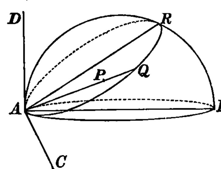
us find the components of the attraction exerted by a uniform hemisphere on a particle at its edge. Let A be the particle, AB a diameter of the base, AC the tangent to the base at A; and AD perpendicular to AC, and AB. Let RQA be a section by a
