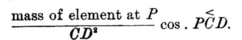
Now suppose the density of the chord AB to be the same as that of the arc. Then for (mass of element at  $P \times \cos P\widetilde{C}D$ ) we may put mass of projection of element
