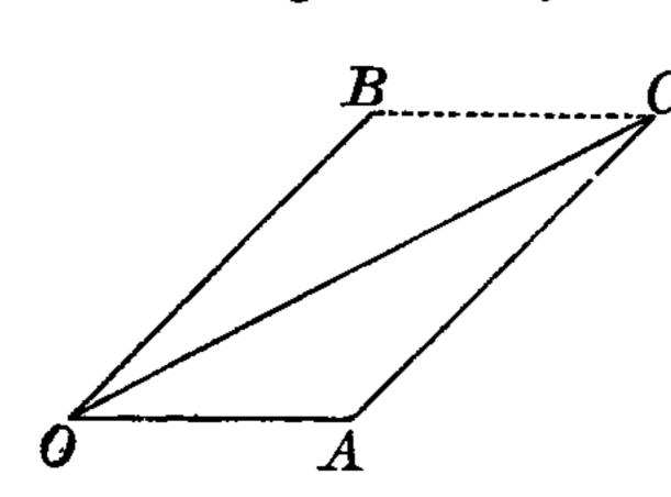
from A draw AC parallel and equal to OB. Join OC:—then OC is the resultant velocity in magnitude and direction.
