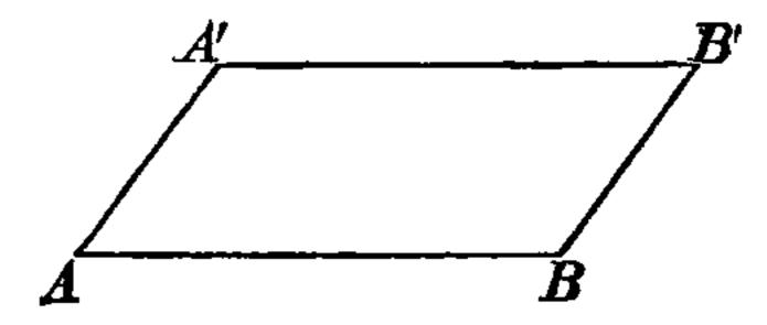
plane without rotation—since, AB being parallel and equal to A'B', we have AA' parallel and equal to BB'; and instead of there being one point of the figure common to both positions, the lines joining the two successive positions of all points in the figure are equal and parallel.
