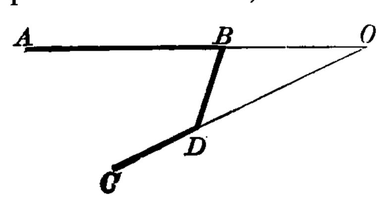
it turned about O. From this it may be easily seen that if the angular velocity of AB be  $\omega$ , that of CD is  $\frac{AB}{OB}\frac{OD}{CD}\omega$ . A.
