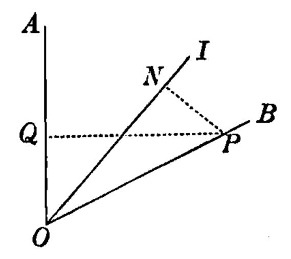
Precessional the actual velocity of the point P is  $\Omega QP$ . But, by the principles explained above, § 99, the velocity of P is the same as that of a point moving in a circle whose centre is N, plane perpendicular to ON, and radius NP, which, as this radius revolves with angular velocity  $\omega$ , is  $\omega NP$ . Hence
