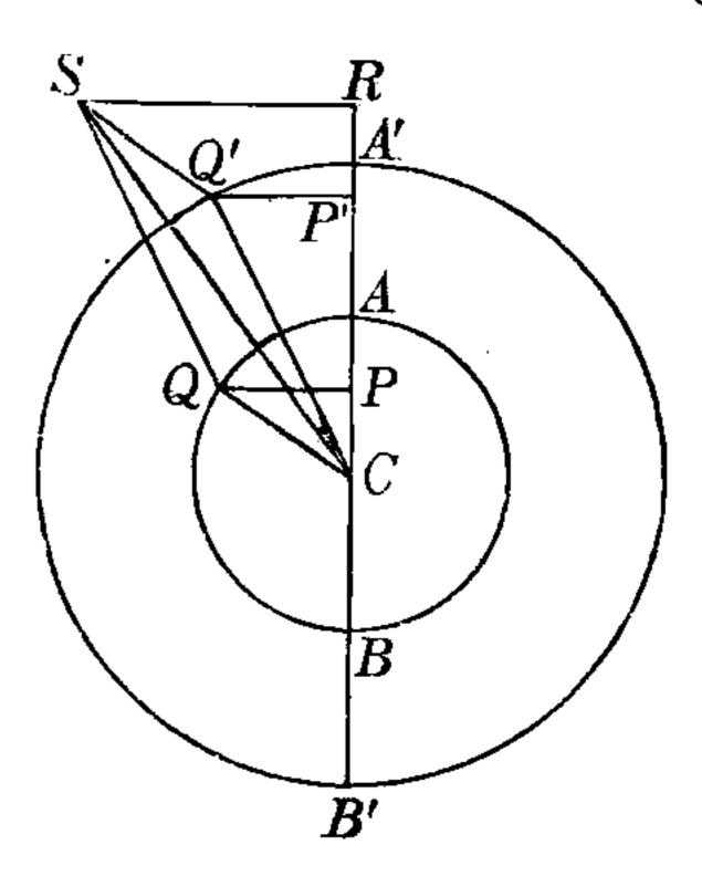
point R executes the resultant of the motions P and P'. But CS, the diagonal of the parallelogram, is constant, and therefore the resultant motion is simple harmonic, of amplitude CS, and of epoch exceeding that of the motion of P, and falling short of that of the motion of P', by the angles QCS and SCQ' respectively.
