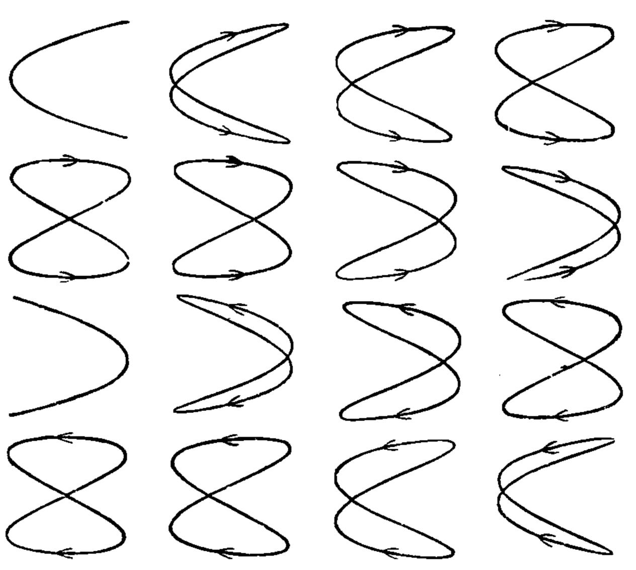
combination of simple harmonic motions of equal amplitude in two rectangular directions, the periods of the components being as 1:2, and the epochs differing successively by 0, 1, 2, etc., sixteenths of a circumference.
