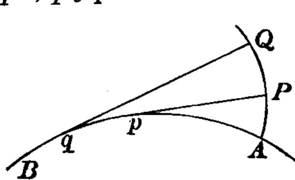
at once that these must be tangents to the arc AB at p and q. Also (see § 90), the string at any stage, as pP, revolves about p. Hence pP is normal to the curve PQ. And thus the evolute of PQ is a definite curve,
