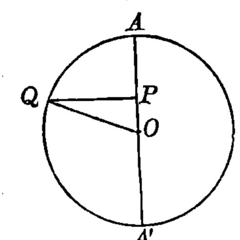
perpendicular QP drawn from its position at any instant to a fixed diameter  $AA^\prime$  of the circle, intersects the diameter in a point P, whose position changes by a simple harmonic motion.
