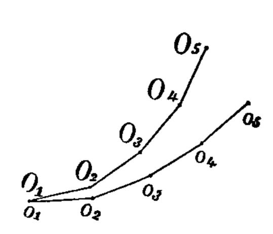
about the latter till  $o_3$  coincides with  $O_3$ , and so on. Hence, if we join  $o_1$ ,  $o_2$ ,  $o_3$ , etc., in the plane of the figure, and  $O_1$ ,  $O_2$ ,  $O_3$ , etc., in the fixed plane, the motion will be the same as if the polygon  $o_1o_2o_3$ , etc., rolled upon the fixed polygon  $O_1O_2O_3$ , etc. By supposing the successive displacements small enough
