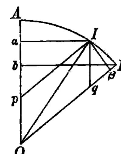
Let the rotations about the two axes be such that that about OB tends to raise I above the plane of the paper, and that about OA to depress it. In an infinitely short interval of time  $\tau$ , the amounts of these displacements will be  $\rho I\beta$ .  $\tau$  and - $\varpi Ia.\tau$ . The point I, and therefore every point in the line OI, will be at rest during the interval  $\tau$  if the sum of these
