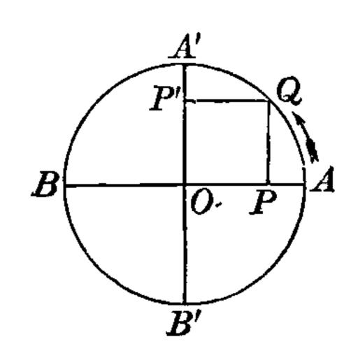
QP'OP is a parallelogram, and therefore Q is in the position of the displacement compounded of OP and OP'. Hence two equal simple harmonic motions in perpendicular lines, of phases differing by a quarter period, are equivalent to a uniform circular motion of radius equal to the maximum displacement of either singly, and in the direction from the positive end of the range of
