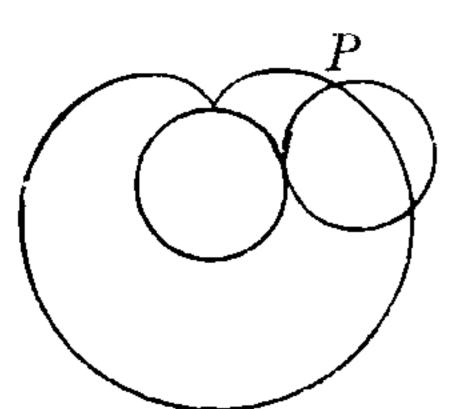
we have already met with examples, §§ 70, 91, and others will be presently mentioned. Of the former, we have in the first of the appended figures the case of a circle rolling externally on another of equal size. The curve in this case is called the Cardioid (§ **49**).
