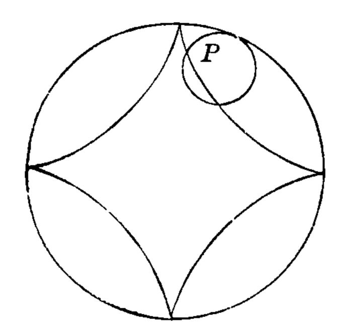
In the third diagram, we have a hypocycloid traced by the rolling of one circle internally on another of four times its radius.
