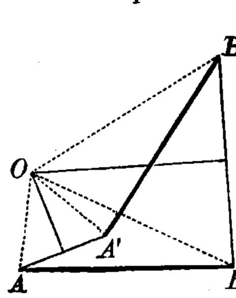
a displacement. The lines AA', BB' will not be parallel, except in one case to be presently considered. Hence the line equidistant from A and A' will meet that equidistant from B and B' in some point O. Join OA, OB, OA', OB'. Then, evidently, because OA' = OA, OB' = OB and A'B'=AB, the triangles OA'B' and OAB are equal and similar. Hence O is similarly
