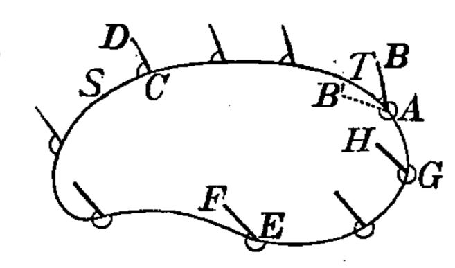
a closed curve as the spherical hodograph; and if A be the point of the hodograph corresponding to them, and AB and AB' the parallels to the transverses, the whole twist in the included part of the bar will be equal to the change of direction all round the hodograph, wanting the excess of the exterior angle B'AT above the angle BAT; that is to say, the whole twist will be equal to the excess of the angle BAB' above the area enclosed by the hodograph.
