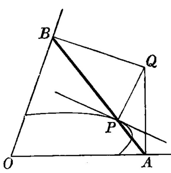
always in two fixed lines OA, OB, any point in it as P describes an ellipse. It is required to find the direction of motion of P at any instant, i.e., to draw a tangent to the ellipse. BA will pass to its next position by rotating about the point Q; found by the method of § 79 A by drawing perpendiculars to OA
