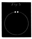
The resonator (fig. 3) is, as in Hertz's experiments, a ring of wire about 70 cm. in diameter, terminating in two balls, the distance between which can be accurately adjusted by means of a screw. The way in which the resonator was used was different from Hertz's method. Two wires of equal length covered with gutta-percha and
