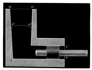
The terminals were composed of L-shaped pieces of ebonite, hollowed out in the manner shown (about full-size) in the figure. Each end of the tube was furnished with a short length of thick rubber tubing, by which the aperture between the glass and the ebonite was closed air-tight. As a further precaution, the space at c c beyond the rubber was filled up by pouring in melted paraffine wax.
