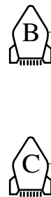
Figure 3. As B and C accelerate, the thread spanning between the midpoints of the ships before the motors were started travels with them, keeping its initial length.
