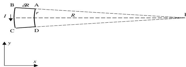
Figure 9: Calculation of the resultant magnetic field  $\mathbf{B}$  at the point  $P$  due to both bound  $\mathbf{B}_u$  and radiation  $\mathbf{B}_a$  components generated by varying currents  $I(t)$  in the loop  $ABCD$
