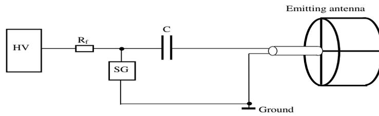
Figure 6: Circuit of the emitting antenna.
