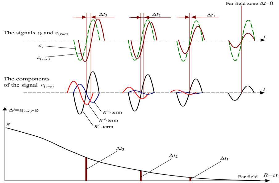
Figure 2: the case  $v = c$ ; evolution (with  $R$  and  $t$ ) of the temporal shift between  $\varepsilon_{v=c}(t)$  and  $\varepsilon_r(t)$ ; specification of the relative contribution of  $R^{-3}$ ,  $R^{-2}$  and  $R^{-1}$ -terms into the resultant signal  $\varepsilon_{v=c}(t)$ ; dependence  $\Delta t(R)$  corresponding to the time shift between instants when signals  $\varepsilon_{v=c}(t)$  and  $\varepsilon_r(t)$  cross zero line
