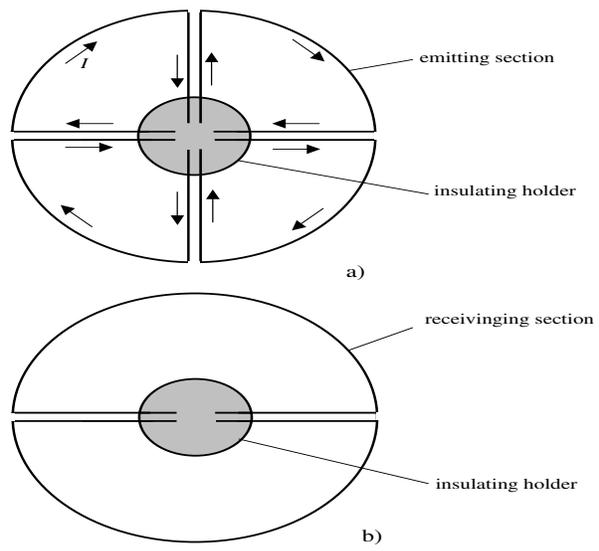
Figure 5: (a) cross-section of the EA; the arrows show the direction of current flows in all sections; (b) cross-section of the RA.
