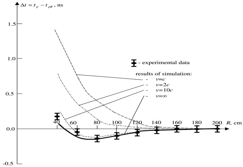
Figure 8: Dot lines illustrate numerical predictions of the dependence  $\Delta t(R)$  for  $v = c$ ;  $v = 2c$  and  $v = 10c$ ; continuous line corresponds to the numerical predictions of  $\Delta t(R)$  for  $v = \infty$ ; empirically found dependence  $\Delta t(R)$  is represented by black circles.
