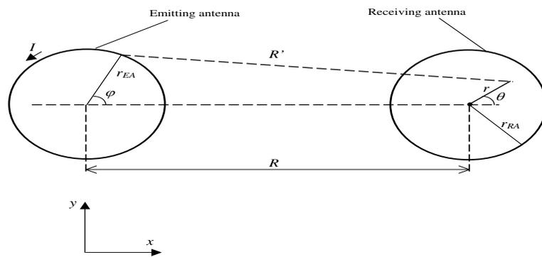
Figure 7: Calculation of the resultant magnetic field  $\mathbf{B}$  and e.m.f.  $\varepsilon(t)$  in the loop of the RA; specification of polar coordinate systems attached to the EA and RA.
