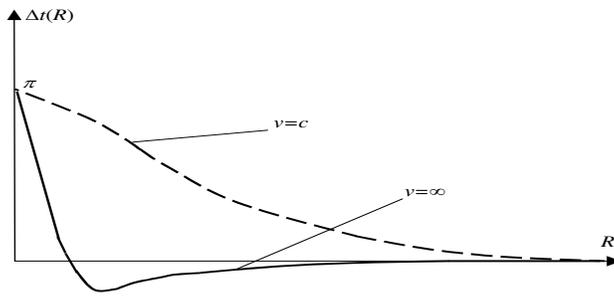
Figure 4: the case  $v = \infty$ ; the dependence  $\Delta t(R)$  is calculated under the assumption that the relative contribution of  $R^{-3}$ -term into the resultant signal  $\varepsilon_{v=\infty}(t)$  is negligible in comparison with  $R^{-1}$ -term at distances  $R > c/\omega$
